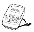
2. Connect printer cable plug cord to the main unit. Arrow (▲) on printer cable plug should face down to main unit.
